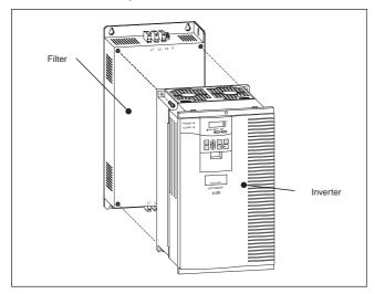
To fix the filter-inverter unit on the back of the cabinet use the mounting bolts provided with the filter. For correct filter performance the filter mounting bolts should electrically bond to the cabinet back panel wich is connected to earth. If this is not possible, the paint should be removed from the cabinet directly under the filter footprint.
